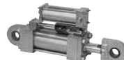
Fig. 200 & C-200 / Fig. 201 & C-201 Hydraulic Shock & Sway Suppressor (Snubber) Size Range: Nine standard sizes with cylinder bores of 1 1/2" to 8" with normal load ratings from 3,000 (LBS) to 128,000 (LBS). All are available with 5", 10", 15" or 20" strokes except the 1 1/2" size which is offered with 5" and 10" strokes only. Snubbers are available with integral or remote reservoirs.
